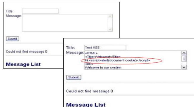
Fig. 2. An Example of injecting a Stored cross site scripting attack.
