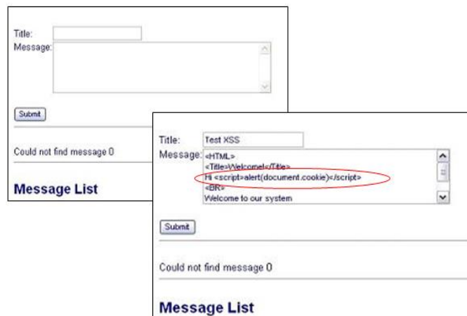
Fig. 2. An Example of injecting a Stored cross site scripting attack.
