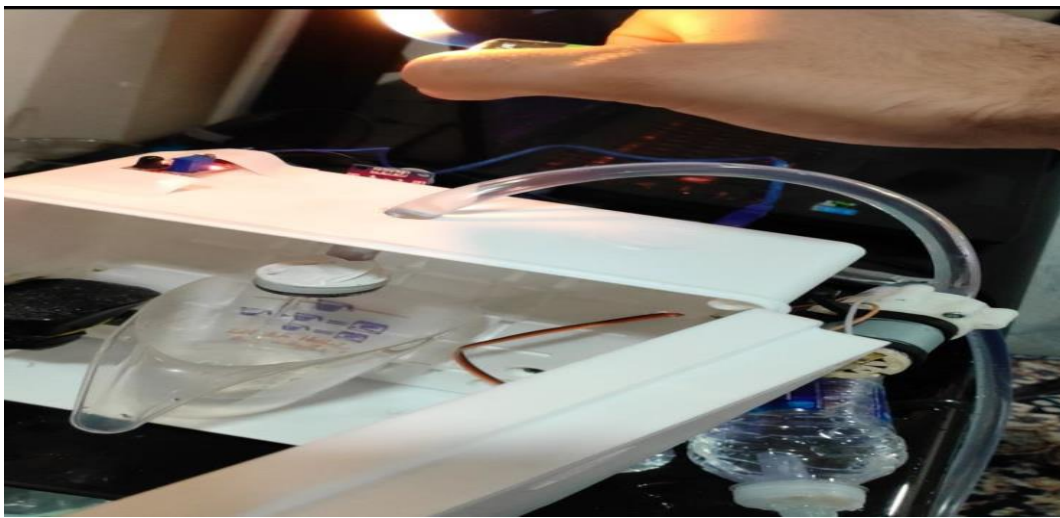
Fig. 6. Operates Water Pump When Detecting Fire.
