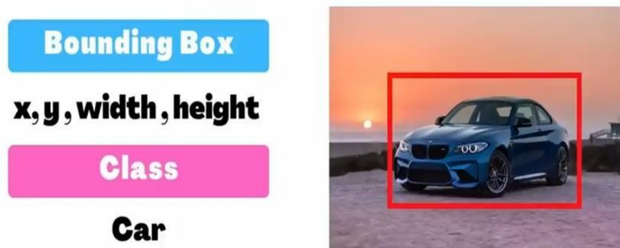
Fig. 2. The main two contents of the object detection process: bounding box and the class.
