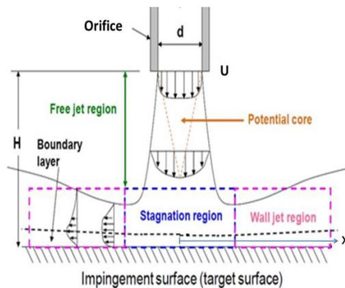
Fig. 2. Characteristic zones in impinging jets [2].
