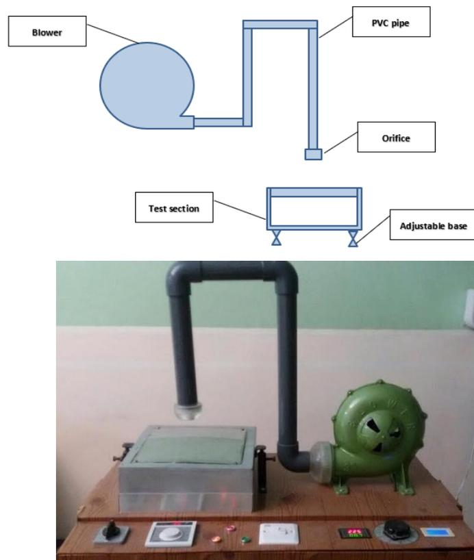
Fig. 3. Schematic and photo of the rig.
