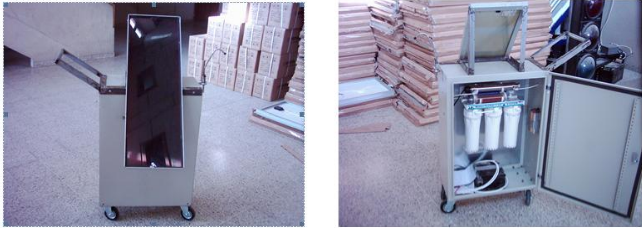
Fig. 3. Solar Desalination and Sterilization System
