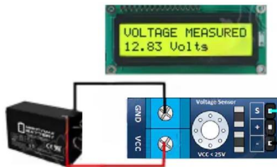
Fig. 3. Module of voltage sensor with example display output
