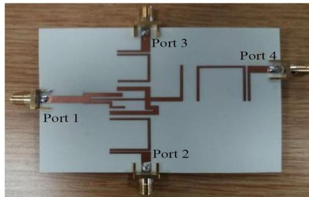
Fig.6. Triplexer Sample
