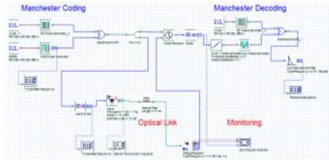
Fig. 1. Manchester coding – decoding system with fiber link
