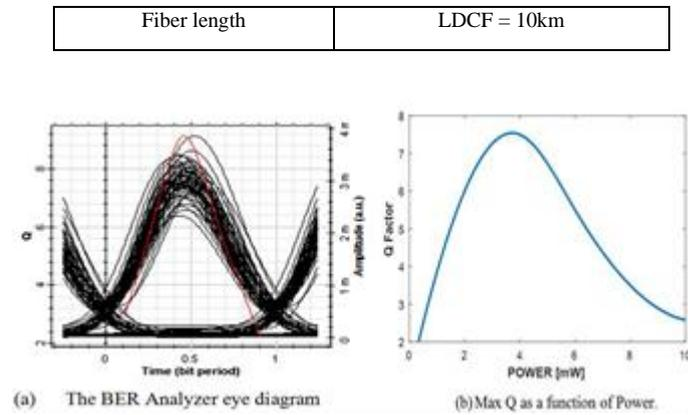
Fig.2. (BER analyzer and max Q factor)
