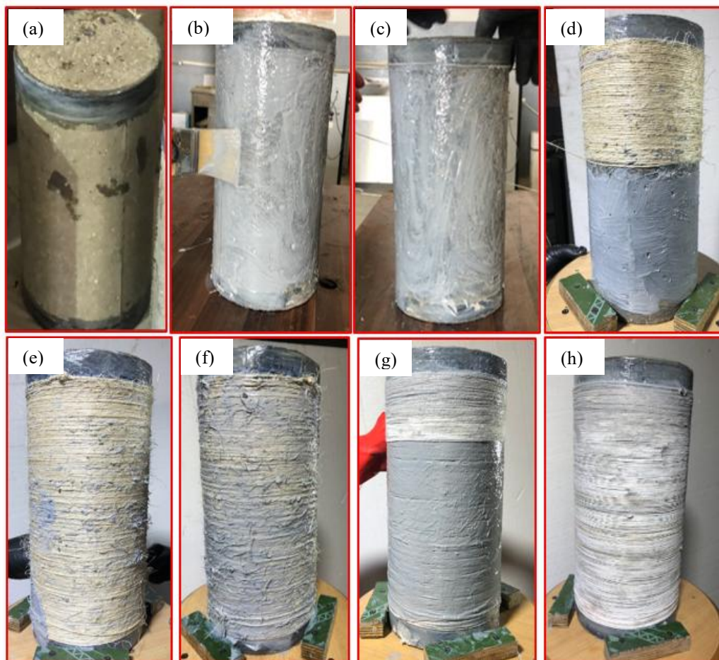
Fig. 5. Steps for applying natural ropes on RC columns for confinement
