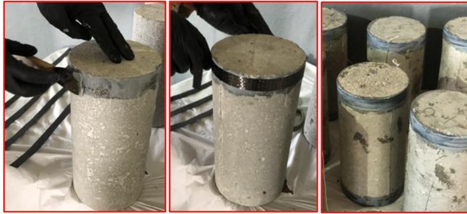
Fig. 4. Adding CFRP strips to both ends of the columns
