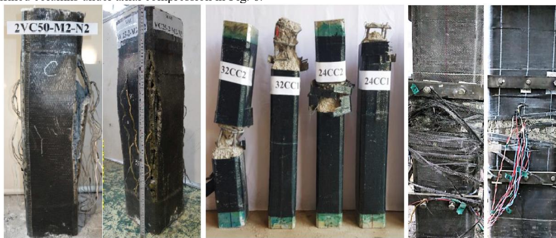
Fig. 6. Columns confined by FRP under axial compression [70 - 72]
