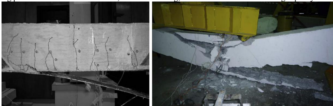
Fig. 4. Failure modes of flexural strengthening [17 & 44]
