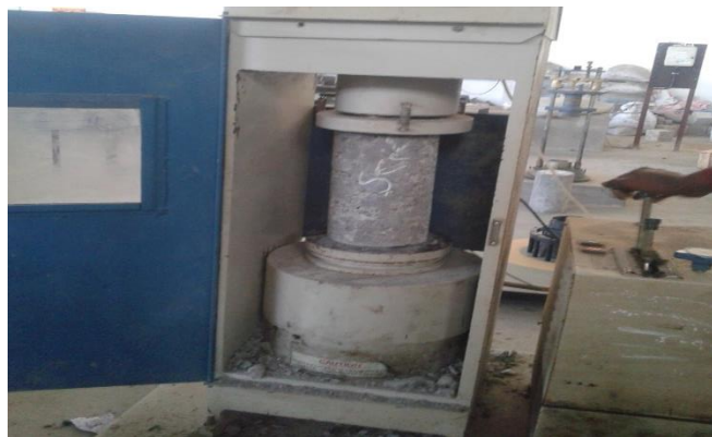
Fig.4. Compressive test on cube
