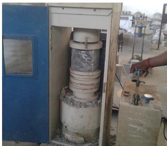
Fig.1. Compressive test on cube
