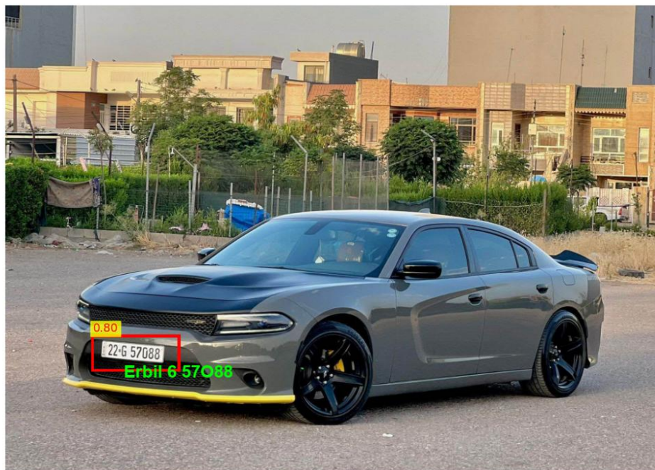
Figure 9: OCR misrecognition of characters: 'G' is incorrectly identified as '6' and '0' is mistaken for the letter 'O', leading to a faulty plate interpretation ("Erbil 6 57O88"). Detection confidence: 0.80.
